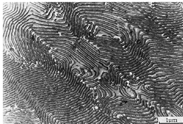
Fig. 6. TEM micrograph of SBM67 ( \Phi_{PS} = 0.67 , M_n = 450 kg/mol) with lamellar morphology (stained with RuO_4 ).
