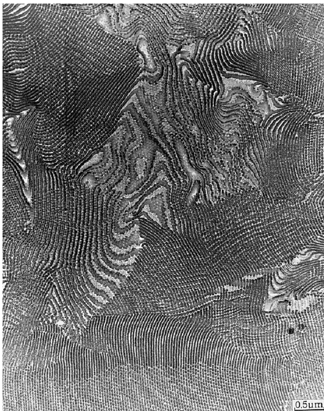
Fig. 5. TEM micrograph of SBM40 ( \Phi_{PS} = 0.40 , M_n = 212 kg/mol) with perforated lamellae of PS. The perforated lamellar structure with parts of the sample cut perpendicular through the perforated lamellae and parts cut through lamellae plane are shown (stained with RuO_4 ).
