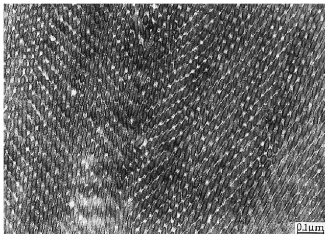
Fig. 4. TEM micrograph of SBM29 ( \Phi_{PS} = 0.29 , M_n = 246 kg/mol) with hexagonally packed PS cylinders (stained with RuO_4 ).
